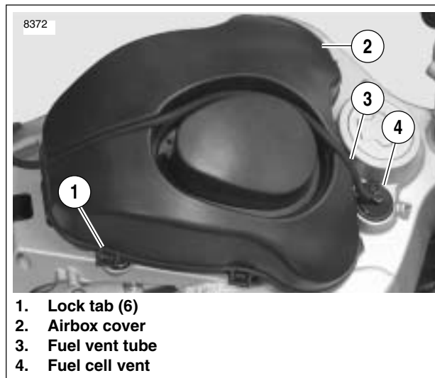
Figure 4-116. Airbox Cover (XB9)
